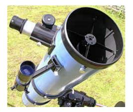
The lockable rack and pinion focuser has a generous 6cm of smooth travel and the 1.25-inch drawtube unscrews to reveal a T-mount camera thread.
